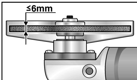
7. Screw the clamping nut (3a), with flange face up, onto the spindle.
