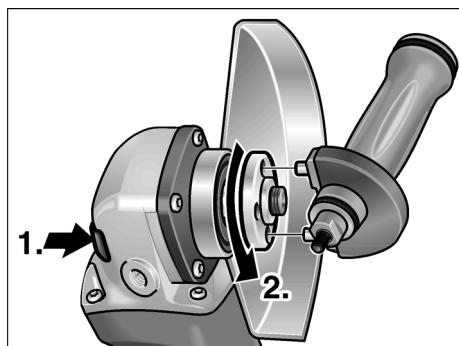
4. Press and hold down the spindle lock (1.).
